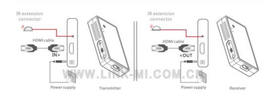
3.Connect the transmitter to the video source device via HDMI cable, then power on the transmitter and video source device.connect the receiver to the video display device, then turn on the receiver &display device, make sure the network and the video connected properly, the LED indicators will light ON.
