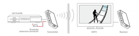
5. When the system working properly, user can use the remote controller of HD player at the HDTV side, the remote controller should be aligned to IR connector of the receiver.
