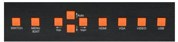
SWITCH: mosaic on/off Vol-: Volume reduce UP HDMI:HMDI input VIDEO:AV input 5<sup>th</sup> . Equipment installation MENU Vol+:Volume increase DOWN VGA:VGA input USB:USB channel 1. Open the package
