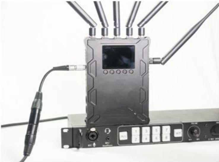
Step1 、 After above connected, power on both Transmitter and Receiver.
