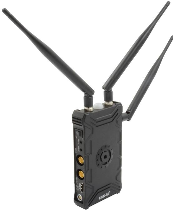
2. On transmitter side, when both SDI and HDMI source are inputted, the transmitter will automatically select the SDI source for transmission
