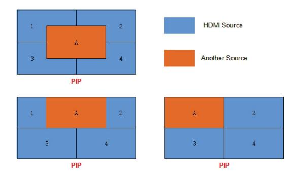
( Under PIP mode, User can use remote control to move the picture A position )
