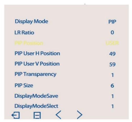
(USER can adjust the PIP position, transparency and size by remote.also can save display mode to 1-9.then next time you can press 1-9 key use saved mode directly.)
