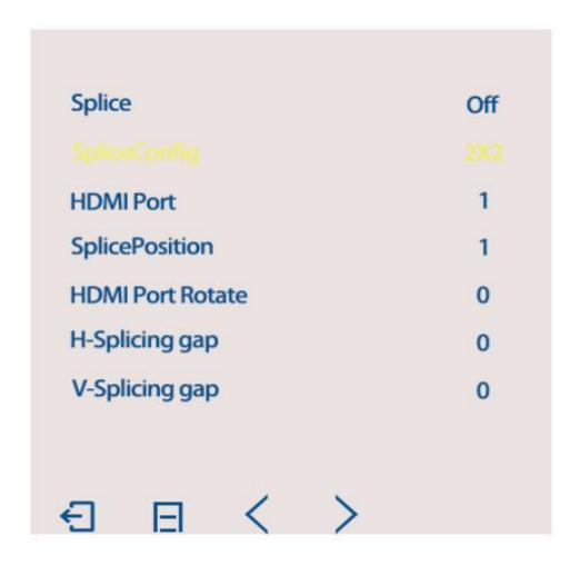
4. Select HDMI port NO. And splicing NO. And adjust according to the prompts in the upper left corner of the screen (for example: 3x3 mode, set the first screen HDMI port to 1 and the Splice Position number is 1, and the upper left corner will show:
