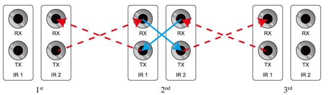
**Note:** the red arrow indicates the two-way 3.5mm infrared 3-section connector; The blue arrow indicates the direction of infrared in the product
